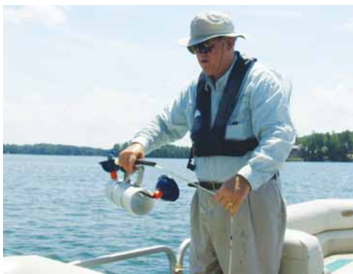
UCR volunteer Woody Williams prepares to deploy a Van Dorn sampler, which is used to collect water samples from different depths in the lake.
