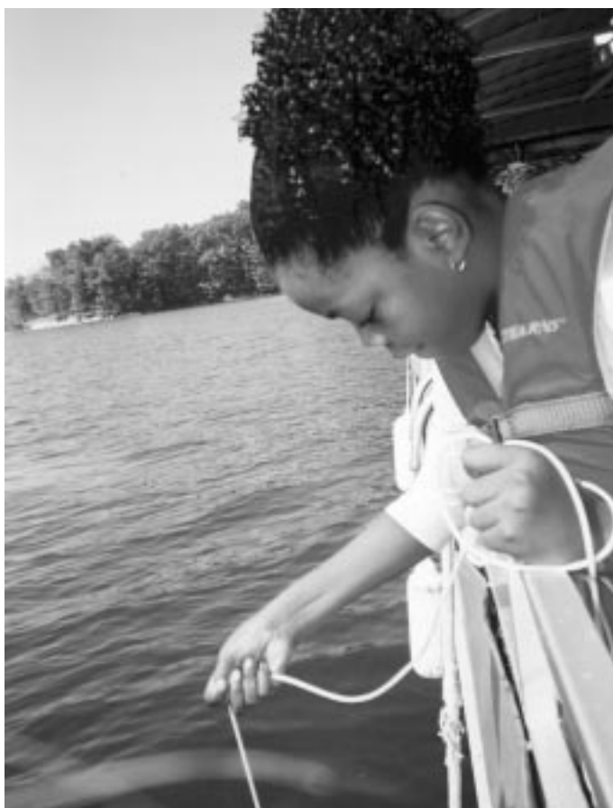
A student tests the turbidity of Lake Lanier using a secchi disc.
